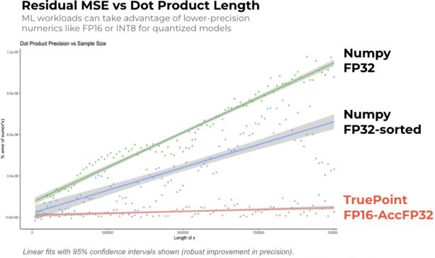
Linear fits with 95% confidence intervals shown (robust improvement in precision). Compares against inputs in FP32 but within the range of FP16 values (remove quantization error effects). Sorted line shows best-case FP32 MSE assuming deterministic compute, like GroqChip™. Compared against FP64 oracle.
